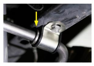
12. Position the Belltech sway bar on the frame mounts with the bar ends angled down pointed toward the front of the vehicle. Fasten the sway bar with the original bolts; hand tighten but do not torque yet.
