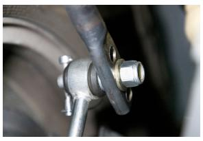
15. Adjust the position of the sway bar so it is centered. Torque the pivot bushing bracket bolts to 45 ft lbs.
